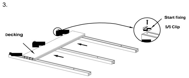
Push the deck planks to the start fixing the S/S Clips
