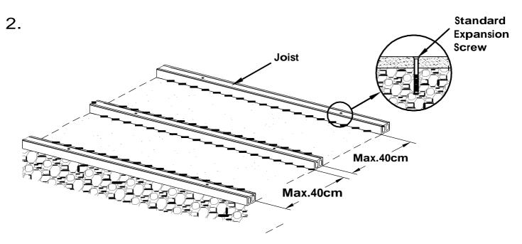
It is recommended that joist span is not wider than 40cm
