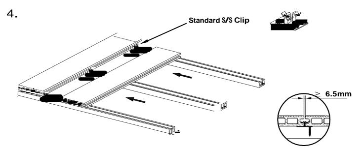
Insert the S/S Center Clip to the decking, fixed to the joist with a screw, then push the next deck plank to the clip
