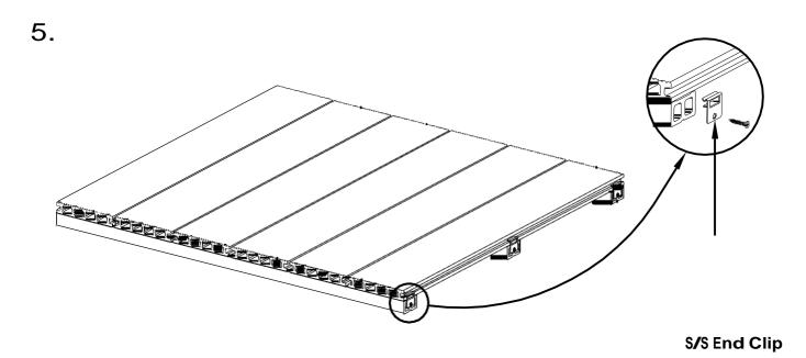
Use S/S End Clip (or Screw) to finish the deck installation
